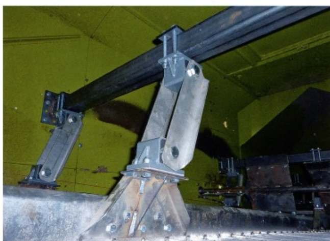
Vibrating element of pumpkin seed harvester 悬架组件在播种机上
