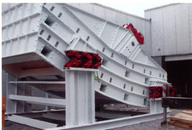
Oscillating mounting at twindeck screen 避震支撑座在双层振动筛上
