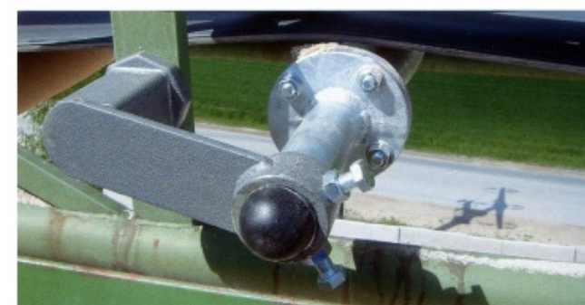
Belt scraper with RESATEC tensioner and special ring lever RESATEC张紧器在皮带刮板上的应用
