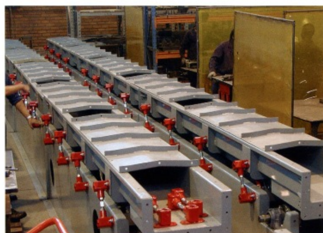
Single deck vibrating feeder with OM elements 振动固定件OM在振动进料器上
